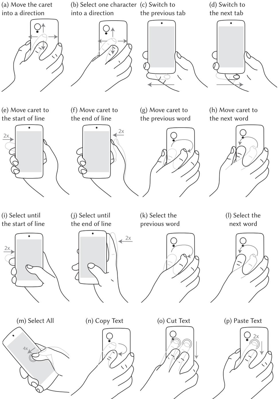
Fig. 4. The gesture set to provide shortcuts for word processing and programming activities. Shortcuts are performed on a smartphone that is capable of sensing touch input on the whole device surface. Gestures for moving and selecting the caret are summarized into one figure for all directions.
