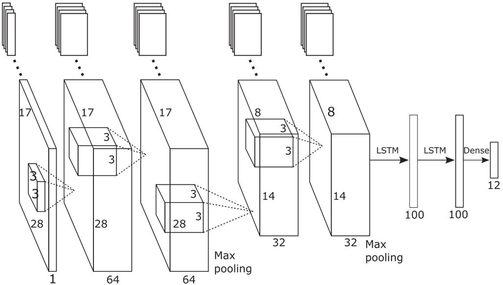
Fig. 7. An illustration of the architecture of our CNN-LSTM model which we used to classify gestures on the FTSP. The first four layers are convolution layers wrapped in a TimeDistributed layer whose output is then fed into two subsequent LSTM layers with 100 units each. The output are 12 values representing the probabilities for each gesture class.
