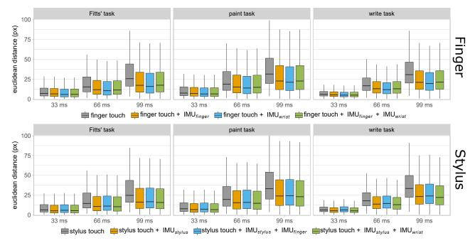
Figure 4. Euclidean distances (*px*) between the predicted and actual touch position for a 33*ms*, 66*ms*, and 99*ms* prediction for finger and stylus input. 10*px* equals to 0.79*mm* and 10*mm* equals to 127.20*px*. Error bars show the 75% quantiles, boxes the 50% quantiles, the black line depicts the median.
