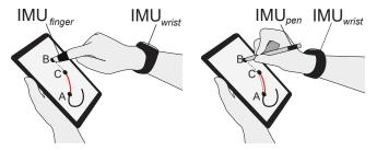
Figure 1. Sketch of *PredicTouch*. Point (A) shows the touch position registered by touchscreens due to latency. Point (B) shows the actual position of finger/stylus. Point (C) shows the touch position extrapolated by *PredicTouch* to reduce the visible latency of touchscreens.
