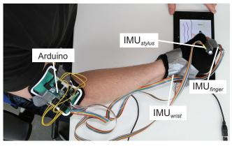
Figure 2. System overview: IMUs at a stylus, the index finger, and the hand wrist are connected to an Arduino board located at the upper arm.
