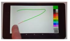
Figure 5. Image of 66 ms touch-only prediction in the painting task. The prediction is exemplarily highlighted by the red line.
