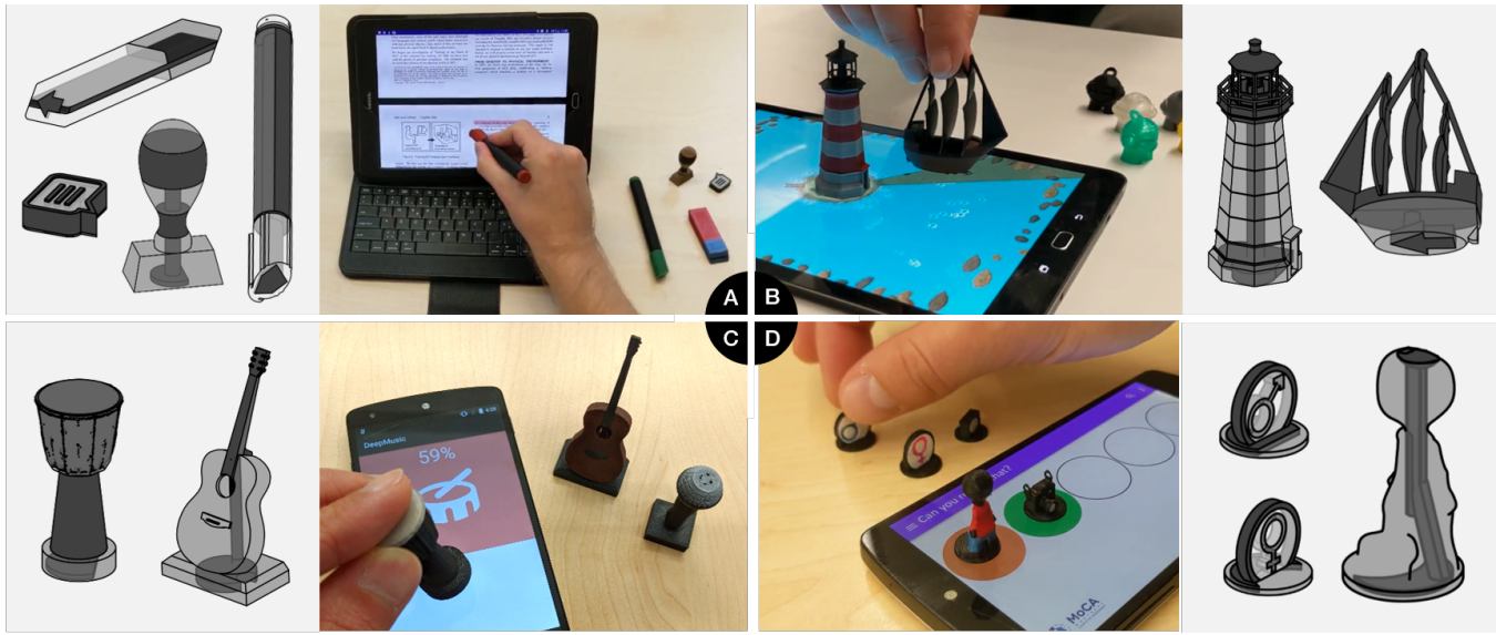
Figure 10: Itsy-Bits enhances editing on small devices involving frequent tool changes (A), makes interactive board games more individualized (B), serves as a mobile mixing console (C), or improves tangible learning experience (D).
