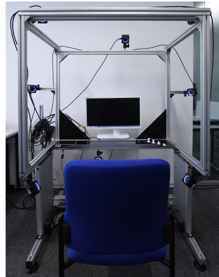
Figure 2. The setup with the 6DOF tracking system, the four pitch stabilizer on the left and the Motorola Nexus 6 with markers.
