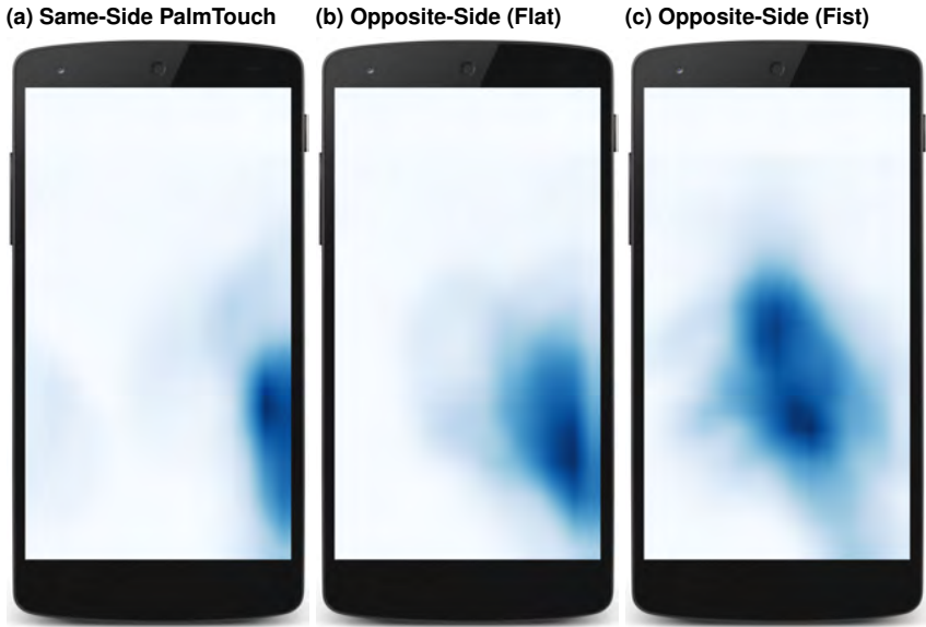
Figure 4.6: Average capacitive images representing the location of the palm touches for (a) same-side, (b) opposite-side using the flat hand, and (c) opposite-side by forming a fist. All images describe the average capacitive images over each participant.
