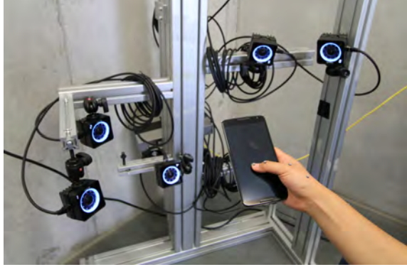
Figure 3.2: Study setup: (a) motion capture system consisting of 8 OptiTrack Prime 13W , (b) reflective markers on a participant's hand, and (c) a participant exploring the comfortable area of the thumb on a Nexus 6 in front of the motion capture system.
