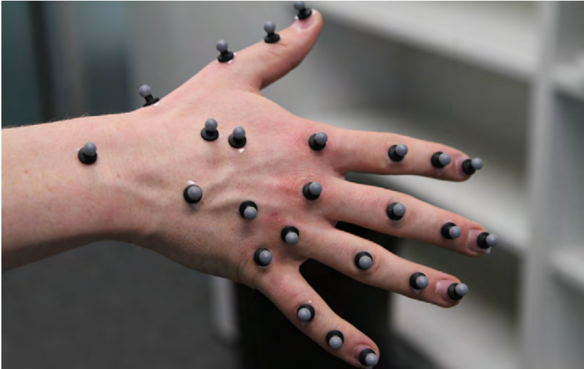
Figure 3.9: Placement of the reflective markers (6.4 mm spheres) on the right hand for enabling motion tracking.
