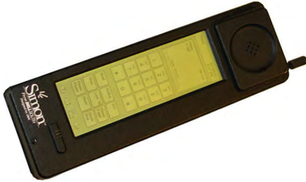
Figure 2.2: Simon Personal Communicator, the first smartphone with a touchscreen by IBM and BellSouth. Image taken from arstechnica 1 .
