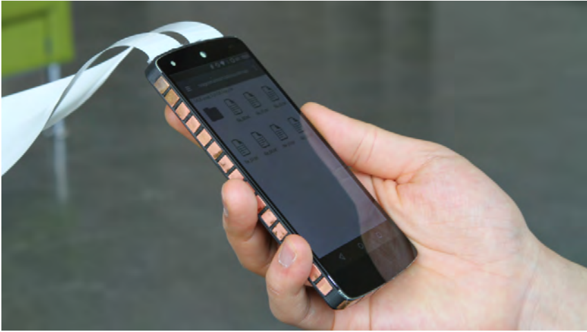
Figure 5.1: Our full-touch smartphone prototype based on two LG Nexus 5 and a Genuino MKR1000 for touch sensing on the edges.
