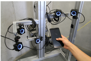
Figure 3: High-precision motion capture system to record finger movements.
