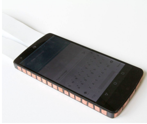
Figure 4: Our smartphone prototype with touch sensing on the whole device surface.
