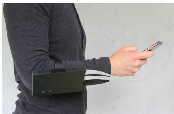
Figure 8: The Hardware Container attached to a participants arm to demonstrate how the prototype can be used in mobile scenarios.
