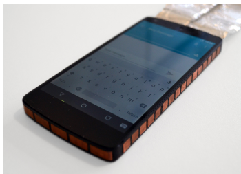
Figure 7: The full-touch smartphone prototype with touch sensing capabilities on the front, back, left, right and bottom side.
