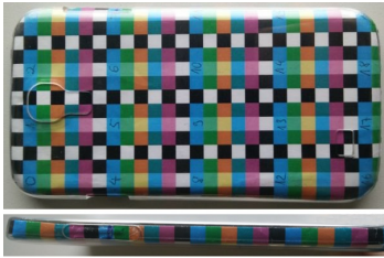
Figure 2: Samsung Galaxy S4 with a colored grid clamped between the phone and a transparent hard case.
