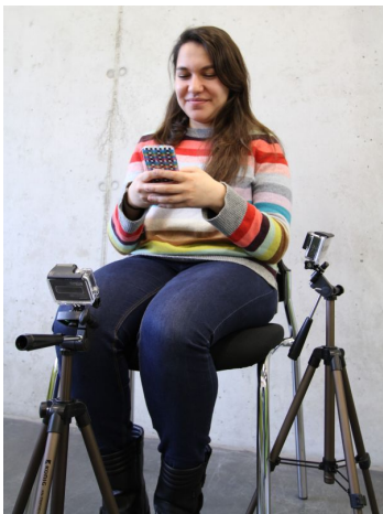
Figure 1: The study setup consisting of two GoPros and the phone with a colored grid.
