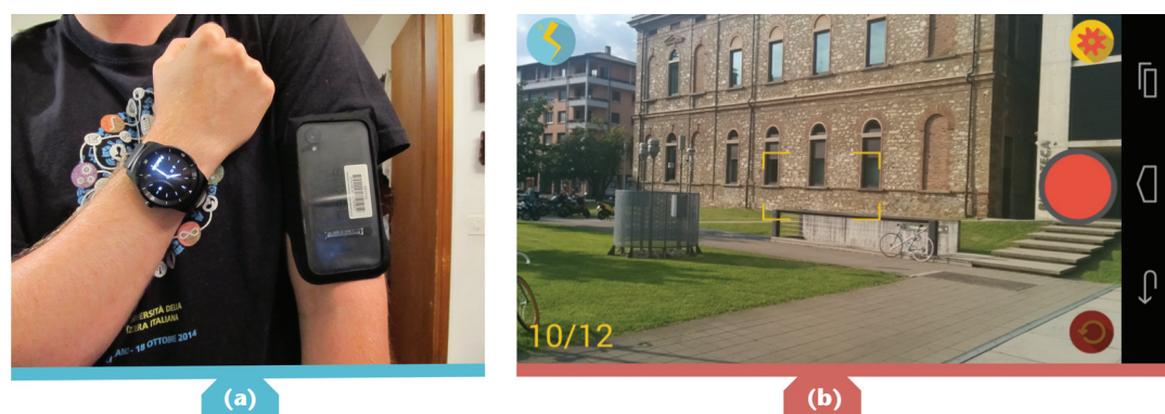
Figure 2. Screenshots of Recall probes for capturing memory cues. (a) The PulseCam prototype hardware. On the left arm, the user has an LG G smart watch for continuous heart rate capture. On the right arm, a Nexus S smartphone is attached to capture the pictures. (b) A screenshot of the My Good Old Kodak application ( https://play.google.com/store/apps/details?id=ch.usi.inf.recall.myoldkodak&hl=en ). The number of remaining photos in the day is displayed in the lower left corner.
