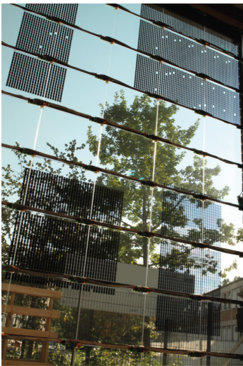
Figure 1: View of the smart window prototype with some transparent and some opaque regions.
